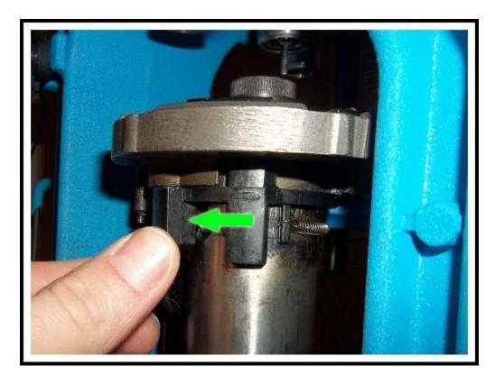
Next while holding the Ring Indexer from spinning raise the platform with the handle to the top of its stroke. (be careful not to pinch your fingers on anything.)
