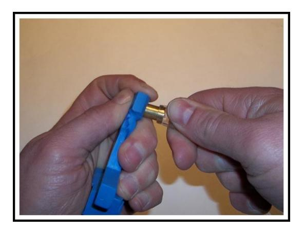
Place your thumb over the top on the brass fitting and hold pressure on it while attaching the hose. The brass fittings are only glued in and this will keep them from popping out while you attach the hose.
